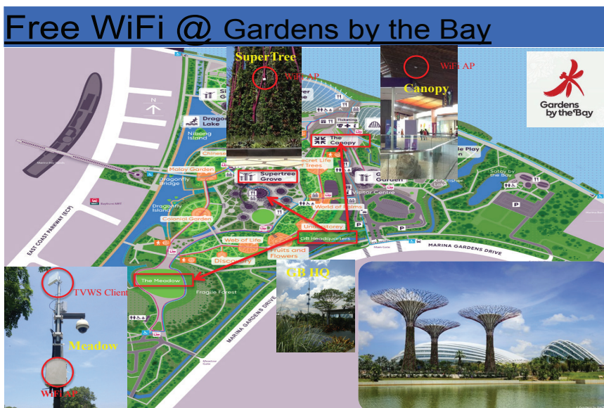
Figure 16: Deployment of WiFi access points and surveillance cameras using TVWS technology at the Gardens by the Bay, Singapore.
