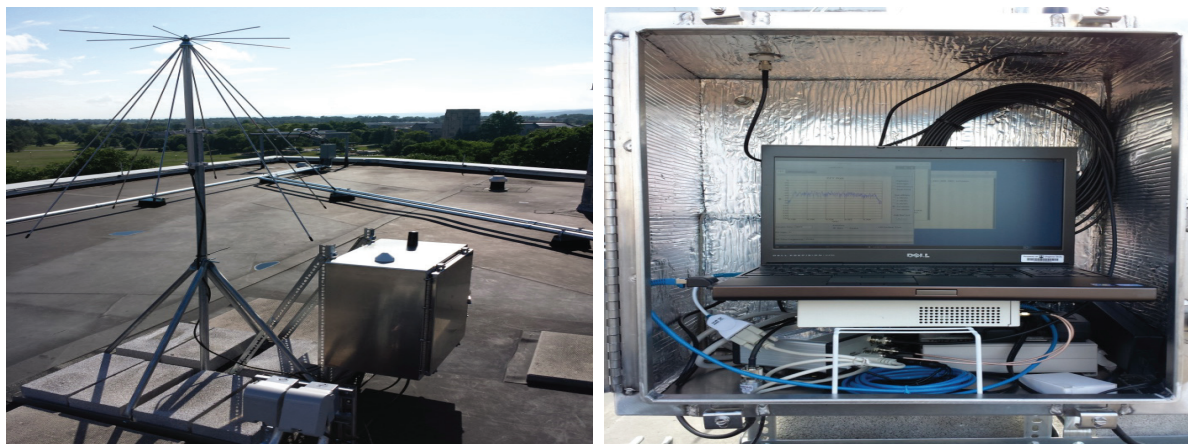
Figure 11: Typical fixed O-CORNET node: mount with antenna and enclosure (left) holding a laptop, N210 USRP with SBX daughterboard, filters and GPS receiver (right).
